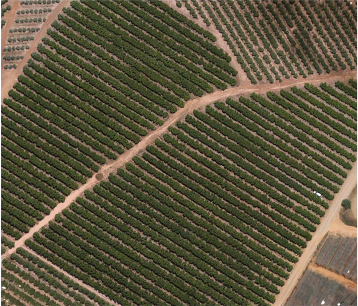
Figure 80. A composite orthomosaic processed by the edge device, effectively merging a sequence of aerial photographs acquired during drone flight operations
